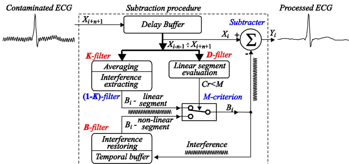
Fig. 1 Generalized structure of the subtraction procedure for power-line interference removal from ECG signals
