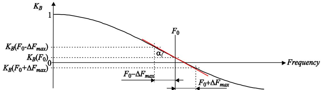
Fig. 2 Linear approximation of the frequency response of **KB**-filter
