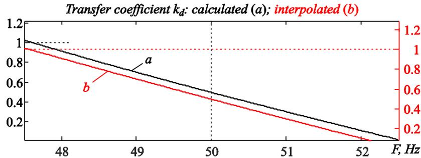
Fig. 3 Linear interpolation of the coefficient  $k_d$  for frequency deviation  $F = 50 \pm 2.5$  Hz
