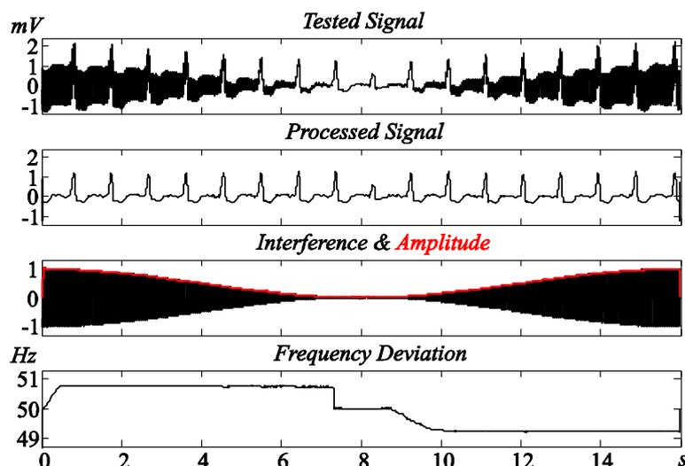
Fig. 7 Experiment with the function (PLinterference\_removing\_Vd2)
