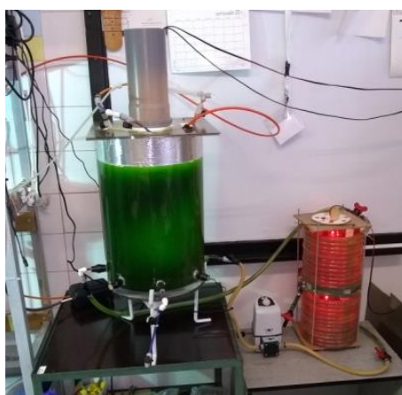
Fig. 4 A hybrid PBR including long tube and stirred tank reactor configuration [41]
